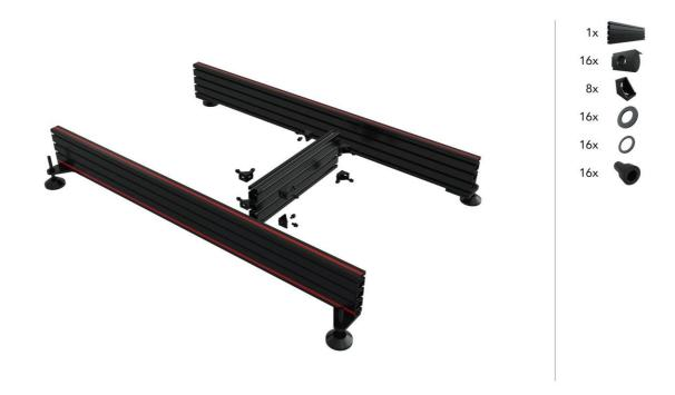
Note: make sure to break off the taps in the corner brackets with a flat screwdriver if they don't sit flush on the aluminium profile as demonstrated here
